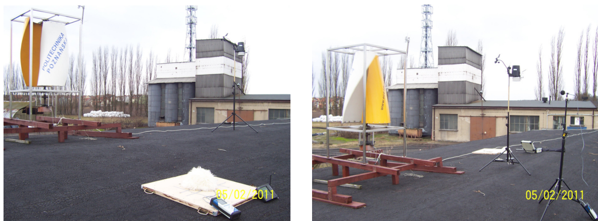
Figure 3. View the location of the measuring microphone: plate and the stand.
